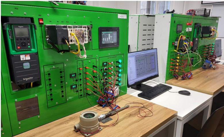
Figure 6– Data collection based on Modicon M340 programmable logic controller
