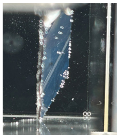
Figure 5 – Gas evolution onto the black-Si photoelectrode at -0.2 \text{ V} RHE in three electrode system in 0.5 \text{ M H}_2\text{SO}_4 electrolyte
