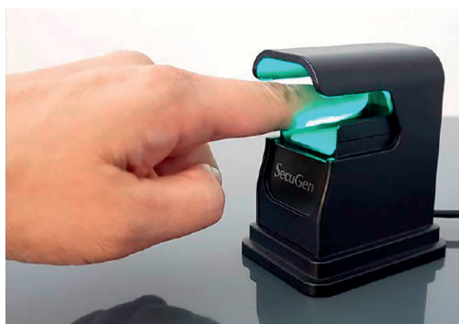
Figure 2 – Hamster Air – SecuGen’s New Contactless USB Fingerprint Reader
