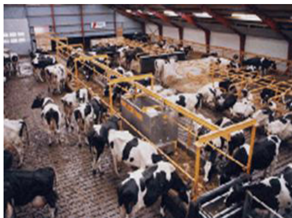
Picture 3 – concentrated feed distribution robot [3]
