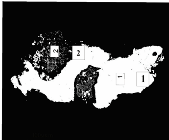
Figure 6 – BSE image showing intergrowth of electrum (1) and native silver (2) with inclusions of high-grade gold
