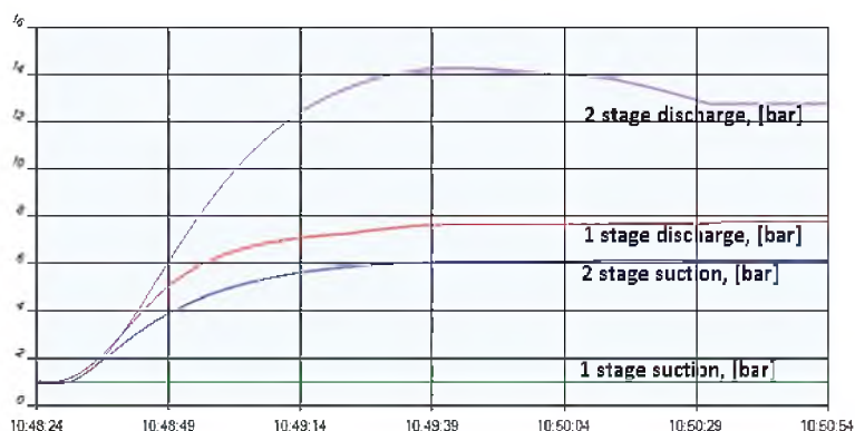
Fig. 6. Pressure of gas during the compressors' start sequence
