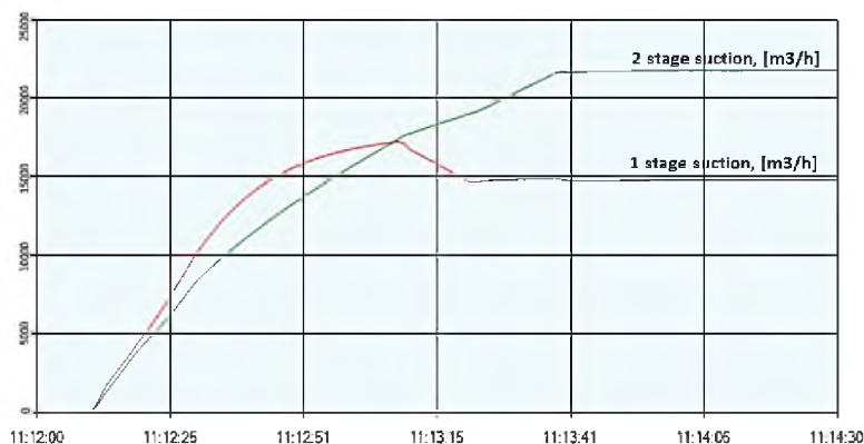
Fig. 5. Volumetric flow-rate of gas during the compressors' start sequence
