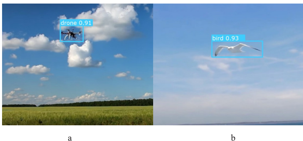
Figure 4 – Inference frames of the trained YOLOv10m model: (a) frame from the DJI F450 flight video; (b) frame of a bird (seagull) flight
