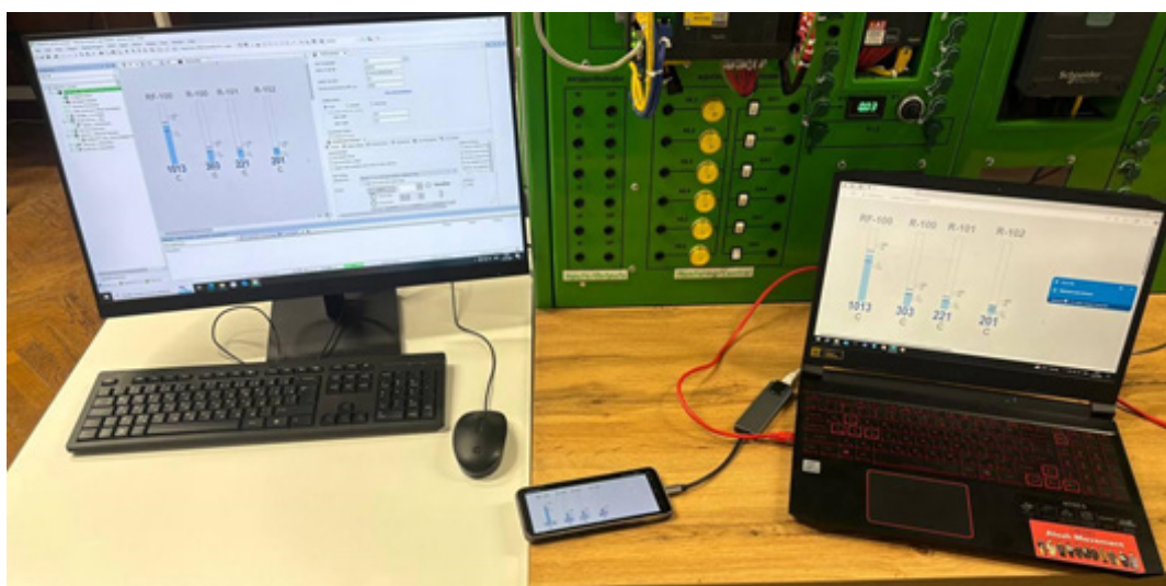
Figure 13 – Mobile PLC Modicon M241 control with Webvisu and EcoStruxture Machine Expert
