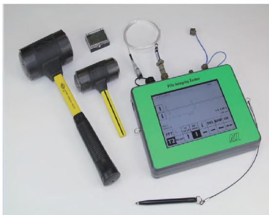
Figure 1. Pile Integrity Tester - PIT-QV
