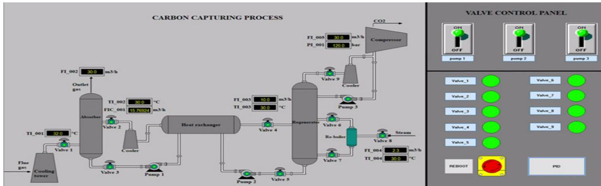
Figure 9 – HMI display for carbon capturing process
