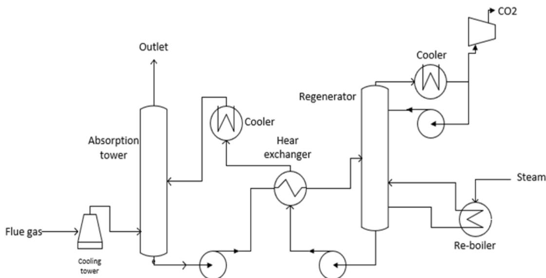
Figure 1 – Technological process scheme of capturing  $\text{CO}_2$
