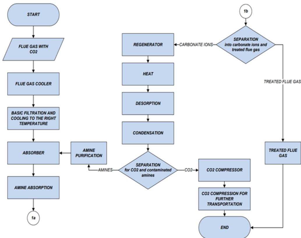
Figure 2 – Sequence of technological process of capturing CO<sub>2</sub>
