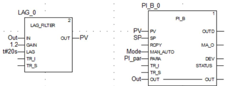
Figure 11 – PID regulator realization in PLC
